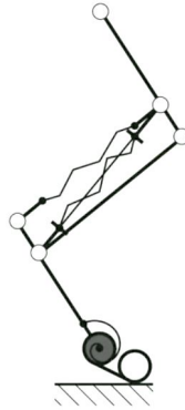
Figure 4. An example of a spring-loaded leg from [10].
