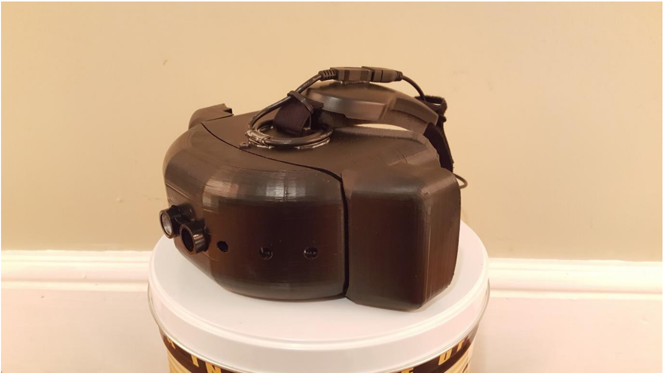
Figure 10. \frac{3}{4} view of prototype showing sensors mounted and speaker side wings.
