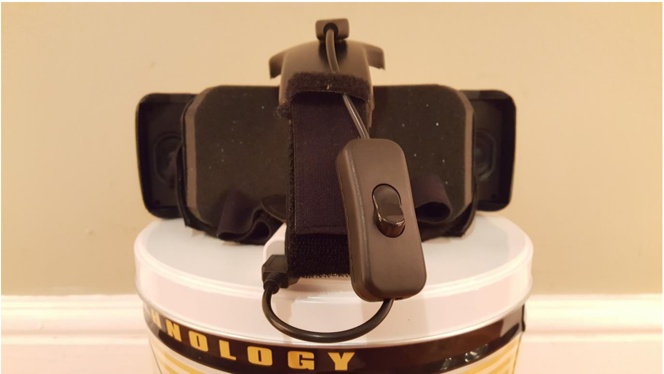
Figure 11. Rear view of LENS system displaying power switch, foam padding, and headstrap.
